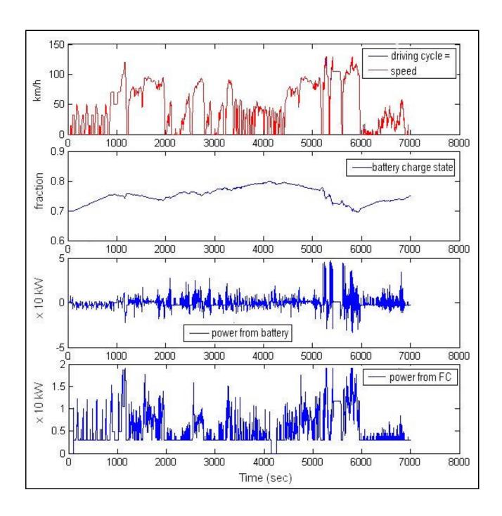
Figure 1. Performance of PEMFC/Li ion battery hybrid car under mixed urban/highway driving cycle shown at top.
