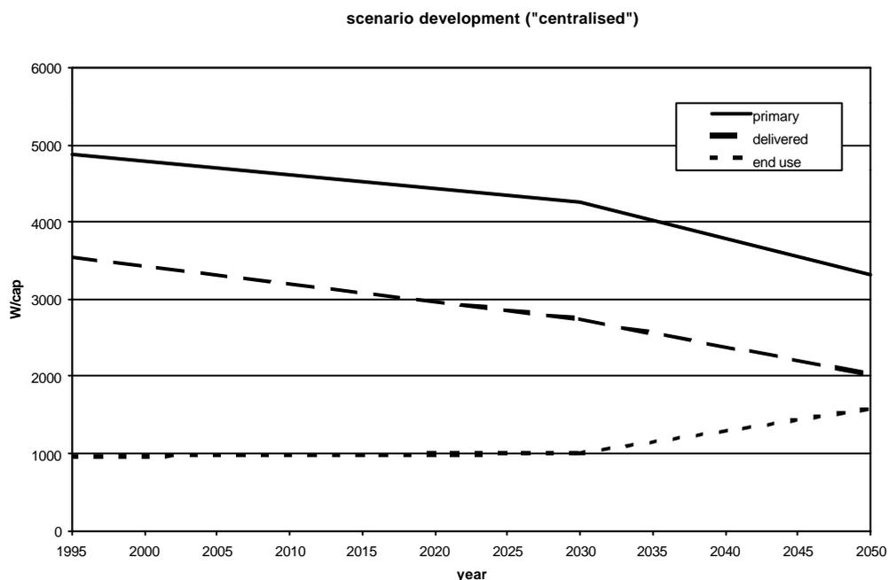
The two figures above show the trends in energy produced, delivered end finally used, for the two lines of scenarios. The development to 2030 is that of the official Danish plan, but from 2030 to 2050 the two scenarios differ: the decentralised scenario has end use growth only in electricity use, whereas the "delivered energy" indicates considerable improvements in end-use efficiency, and the
