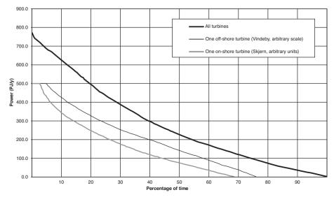
Figure 1: Annual wind power duration curve (percentage of time the wind power production exceeds a given value) for Denmark, for one onshore turbine, for one offshore turbine, and for a system with turbines all across the country. All three curves assume the same total rated turbine power (from Sørensen: Renewable Energy, Elsevier 2004).
