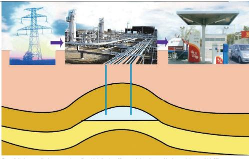
Figure 2: Underground hydrogen store in aquifer, with indication of front-end electrolyser and hydrogen piping to vehicle filling station (from Sørensen: Hydrogen and Fuel Cells, Elsevier, 2005).
